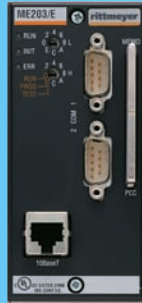
RMME203.E Processor 386/33MHz 8MB RAM
