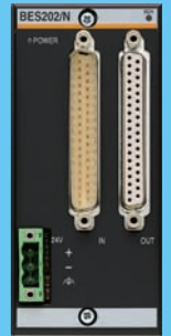
RMBES202.N Bus Extension Slave max. 0.5m power pack 17W
